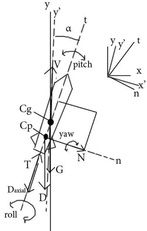
A stable rocket will continuously try to correct its course and return to  $\alpha = \text{zero}$ . However, if the  $\alpha$  increases too much, the  $C_p$  will move upwards and could meet or overtake the  $C_g$ , which will negate the corrective motions entirely, and make the rocket unstable.
